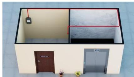
The pipe then rings the hoistway locating several sample points inside, before penetrating back out of the hoistway and back into the equipment room where the pipe run ends with a test point. The exhaust of the air sampling smoke detector is then ran back into the hoistway.
